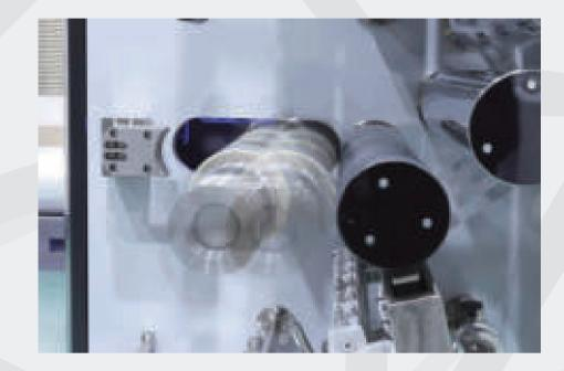
REWIND SHAFT'S HORIZONTAL MOVEMENT CONTROL WITH A LINEAR DRIVE SYSYEM
